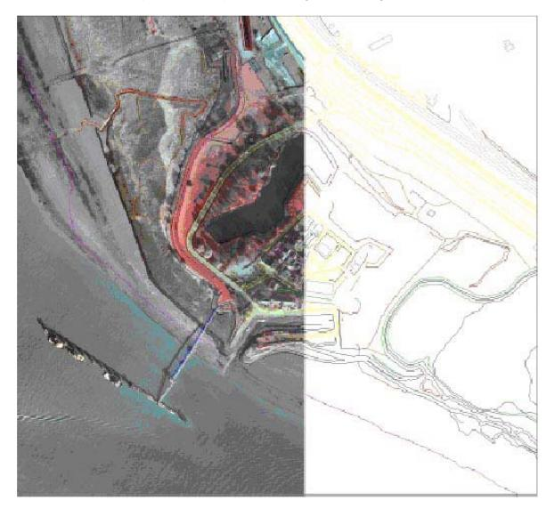
Photogrammetric restitution of the stereo images (60/30% overlap) allowed the DTM creation. The digital processes needed a lot of data control in order to comply with quality criteria of both the DTM and the orthos. The orthos were subject to further radiometric corrections in order to make a homogeneous image representation of the river.
