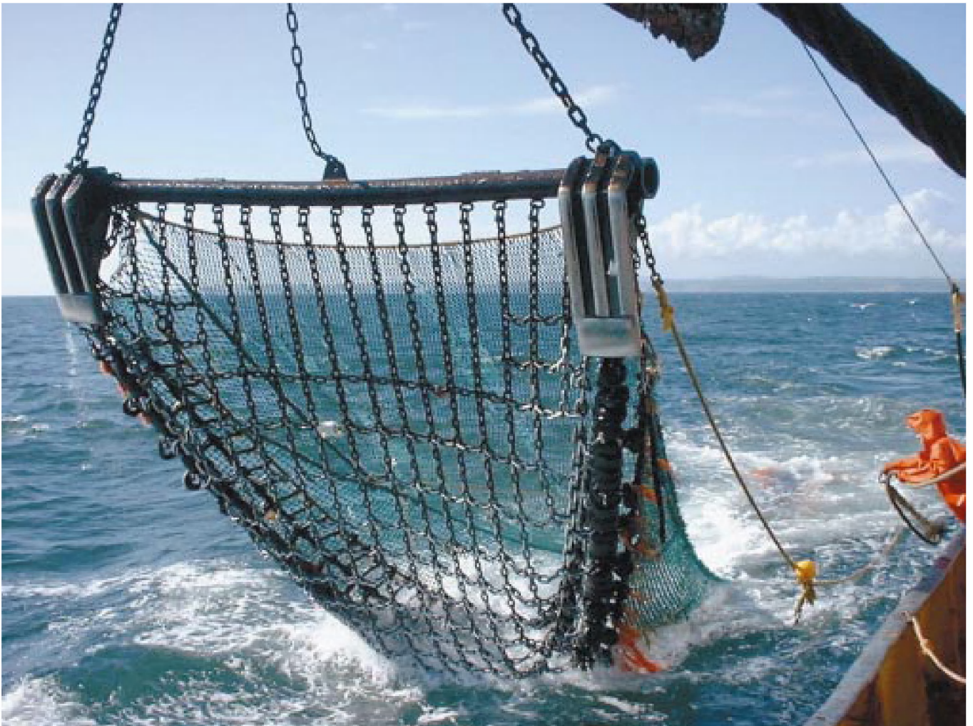
Hauling in a beam trawl, showing the skirts enabling the net to be trawled on the seabed. Spike Searle
