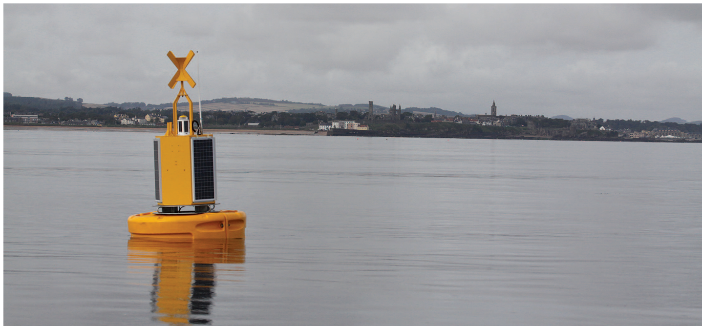
Figure 4.4. PAMBuoy is an example of a passive acoustic monitoring system mounted on a moored or drifting buoy that measures marine sounds and carries out acoustic detection and classification of different preprogrammed sound sources. It transmits these in near-real time by cell phone or satellite phone networks to base stations, including cell phones. Source: Sea Mammal Research Unit, University of St. Andrews (see http://www.pambuoy.co.uk/ ).
