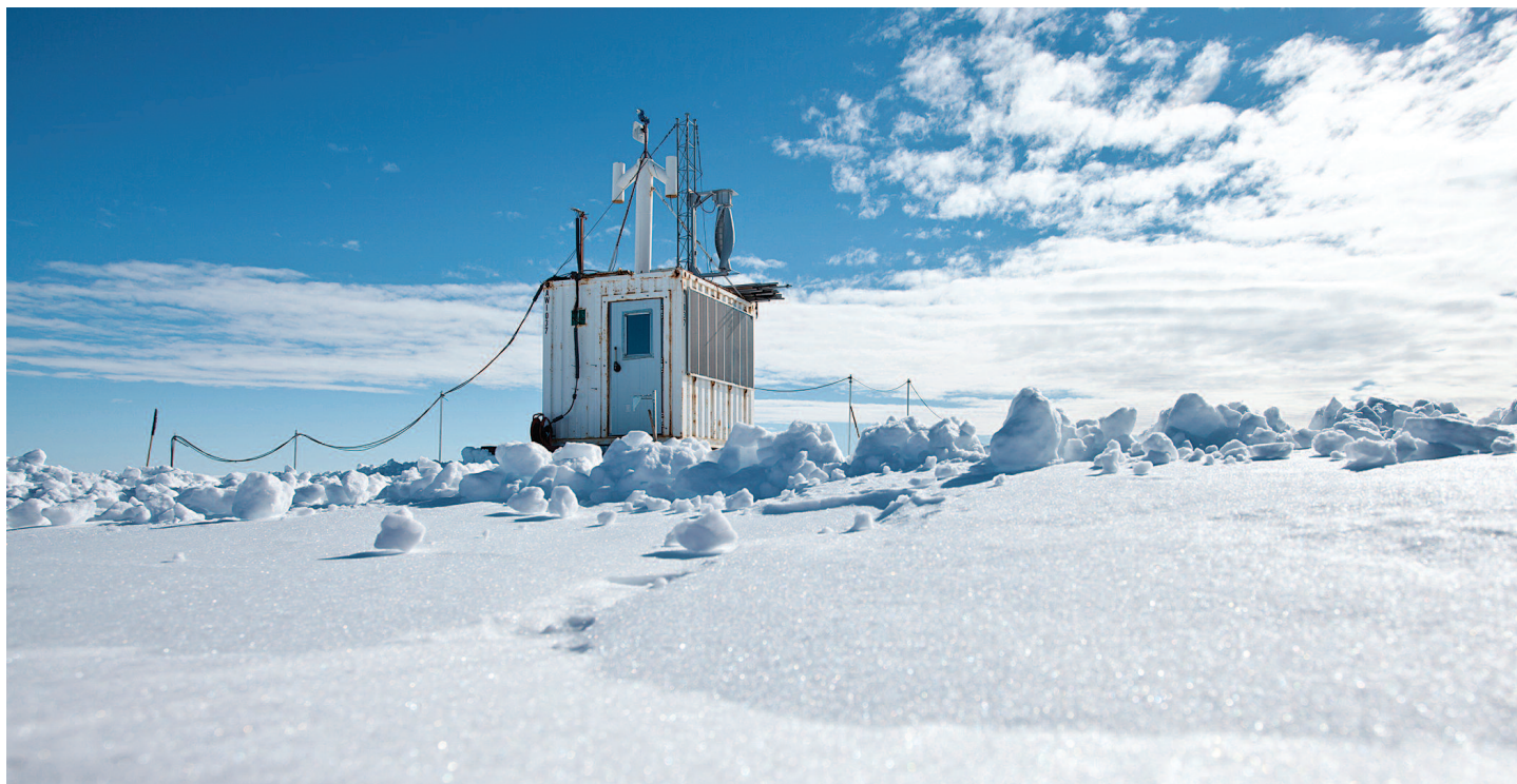
Figure 5.4. The Perennial Acoustic Observatory in the Antarctic Ocean (PALAOA) continuously records the underwater soundscape near the ice shelf edge, 12 km from the German Neumayer-Station III. Photo: Thomas Steuer, Alfred-Wegener-Institut (see http://www.awi.de/fileadmin/user_upload/News/Press_Releases/2013/3._Quartal/Buckelwale_Ilse/2011Palaoa_TSteuer_p.jpg ).
