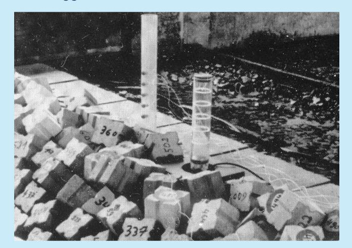
Pressure cells in a first mast registered water pressures caused by wave overtopping at different levels above the foundation. A second mast in the model was connected at the foundation with a leaf spring (with strain gauge) to measure the moment at the bottom of the mast.
