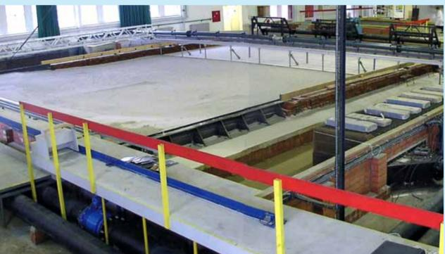
Extensive 2D and 3D model tests proved that the combination of cross-shore wave attack and longshore tidal current is responsible for the continuous erosion at the beach of Knokke-Zoute. Also
