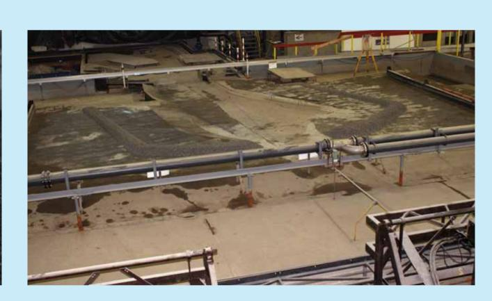
For the design of a new port entrance, measurements in a 3D physical model were combined with calculations of numerical models to obtain the most accurate results for the wave penetration into the port.
