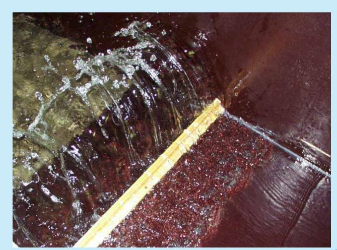
a new sea dike was optimised based on many overtopping tests in the large wave flume. The overtopping discharge in storm conditions was measured and evaluated.
