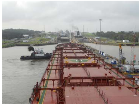
Figure 4. Bulk carrier pushed by tugs to the approach wall before entering Gatún Locks, Panama Canal.
