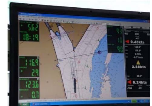
Figure 6. ULCC approaching the Berendrecht Lock, Port of Antwerp, Belgium, assisted by a portable pilot assistance system.
