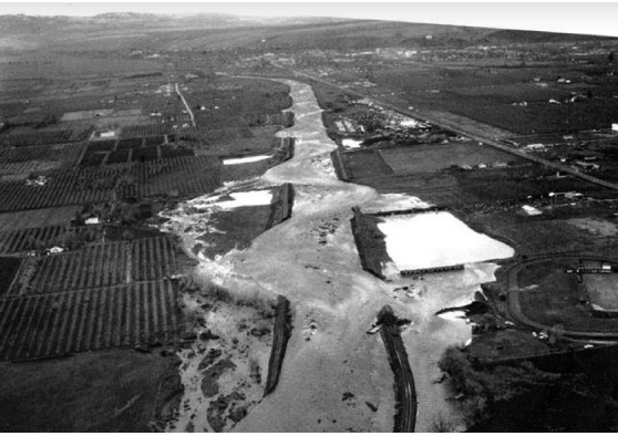
Figure 3 – Aerial view of the Walla Walla River, Washington. The river was straightened between two dykes, but during a flood in 1965 it broke through these dykes, reasserting a meandering pattern. (Photo courtesy of the US Army Corps of Engineers)
