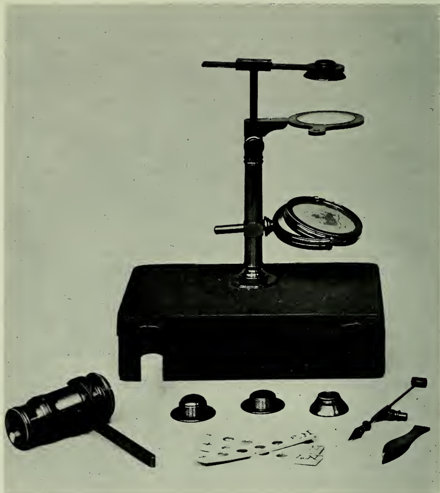
FIG. 13. Ellis Aquatic Microscope, Inventory 1911-294, in the Science Museum, London. The Museum description states: "This type of microscope may be regarded as the precursor of the most complete and perfect of our simple dissection microscopes, and it was made with slight modifications by all the leading opticians until the early years of the 19th century. . . . The round hollow pillar screws into a socket in the lid of the fish-skin case. The mirror mounted in gimbals is fitted to the pillar by a spring-pin and socket. The inner sliding rod which carries the objective arm can be fixed at the desired height by a clamping screw. The stage is removable for portability, and a Wilson screw barrel microscope with three additional powers is added, which can be adapted to the stand". (Photograph British Crown Copyright. Science Museum, London.)
