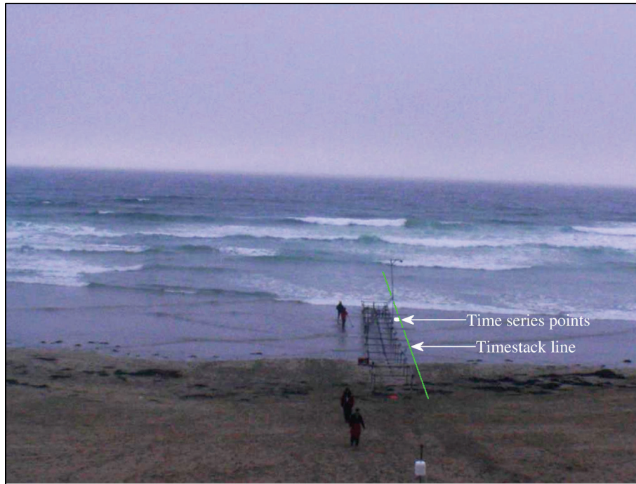
Figure 5.3: Example image of the video collection, including location of pixel intensity time series points and timestack transect. Image brightness and contrast was enhanced compared to raw image for increased visibility.
