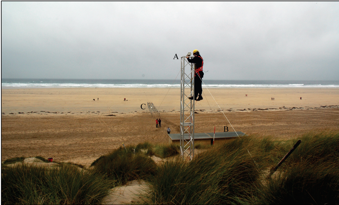
Figure 3.7: Overview of the BeST field location displaying camera tower (A), data logging cabins (B), instrumentation scaffolding (C).
