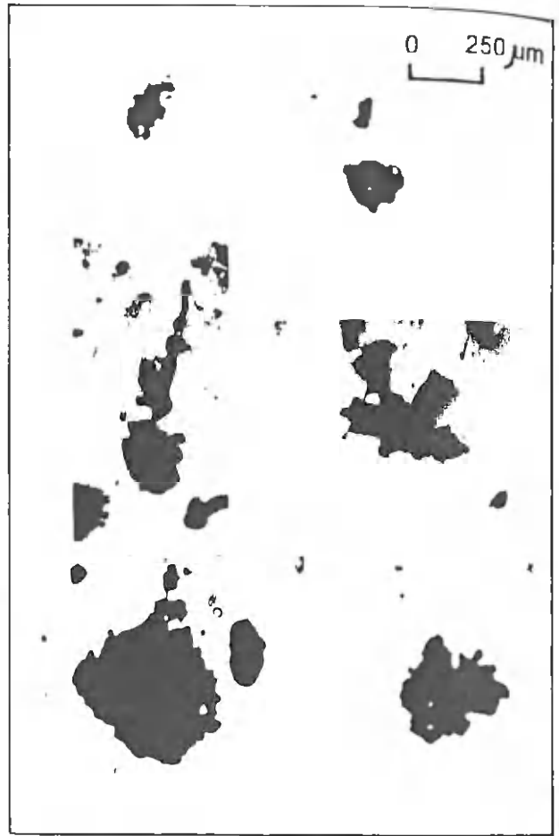
Fig. 7. In situ photographs of flocs in the Dollard estuary. Those with 'stringers' were photographed around slack tide.
