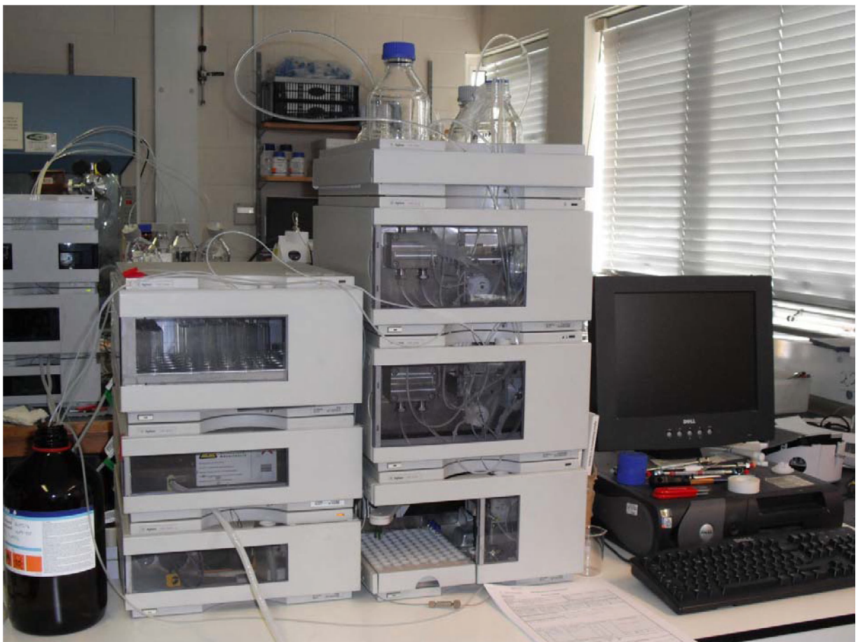
Figure 5: Agilent system diode array detector and pumping system for High performance liquid chromatography.
