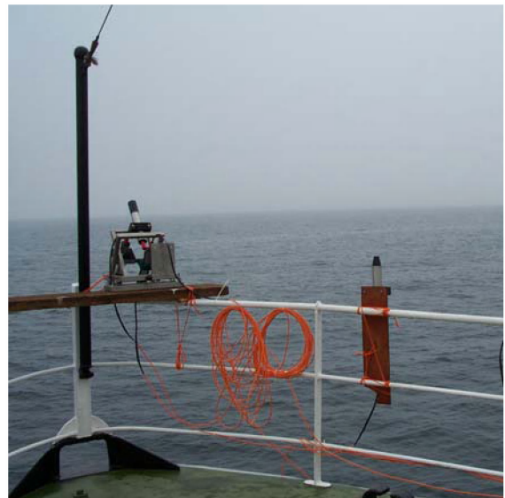
Figure 10. (left) System of two radiance and one irradiance sensor installed on steel frame. (right) As installed at prow of ship with irradiance sensor mounted separately to reduce optical interference from mast.
