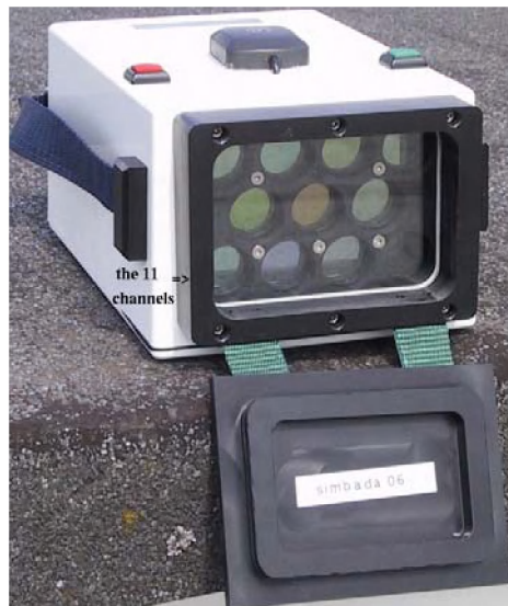
Figure 11. View of SIMBADA showing foreoptics.
