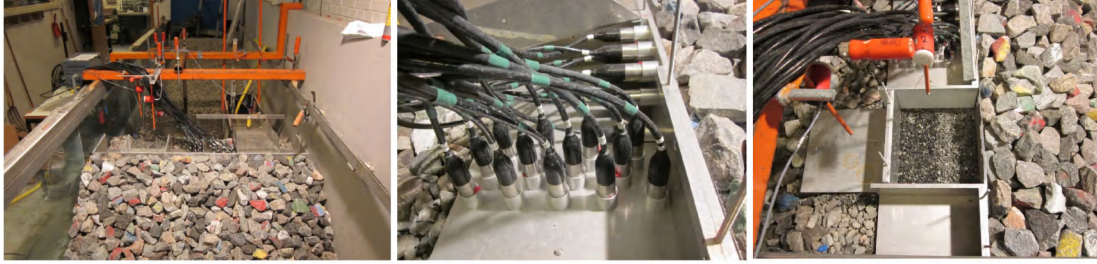
Figure 6. (left) Front view of breakwater, (middle) Pressure transducers in static part of crown-wall, (right) Moveable part of crown-wall.
