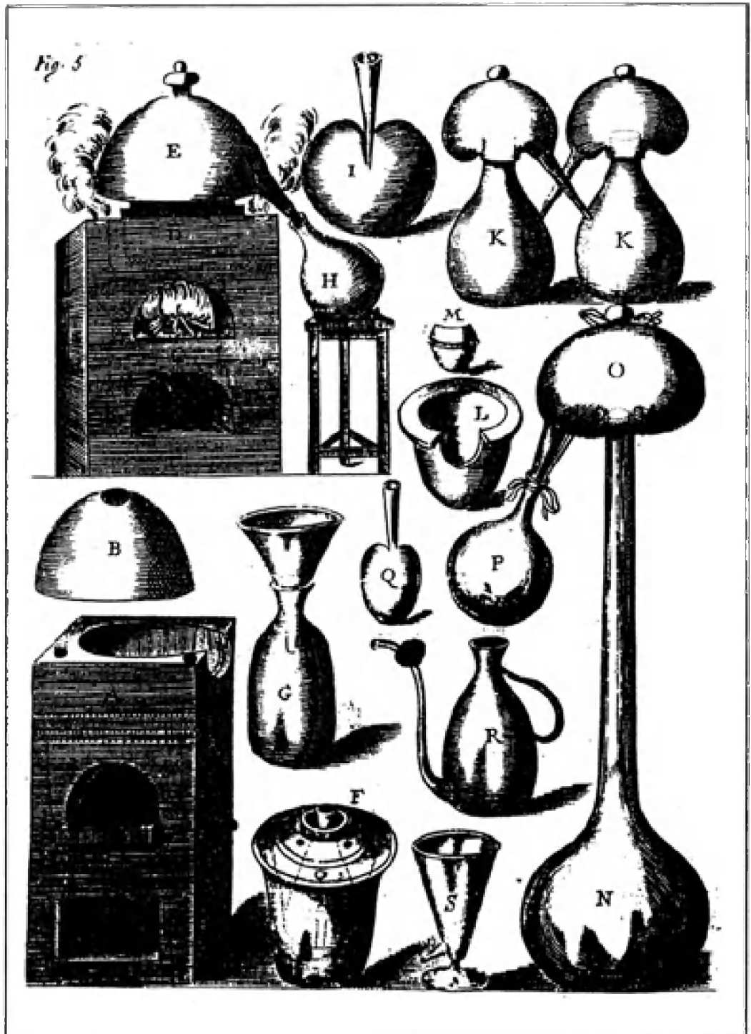
Fig. 36: Equipment used for the production of Oil of Amber and Salt of Amber, from Charras (1678).
