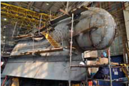
June 2011: the 'bulb' of the ship
