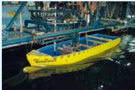
spring of 2011: Damen Shipyards finishes the design and conducts stability tests with models
