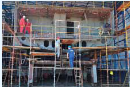
June 2011: bow with cabins for scientists and the bow thruster room
