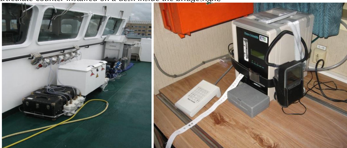
Figure 3. Picture of the sampling equipment deployed onboard; the front of the Belgica's bridge with the denuder, the HiVol and low volume aerosol samplers (left), the BC monitor and particulate counter installed on a desk inside the bridge(right)
