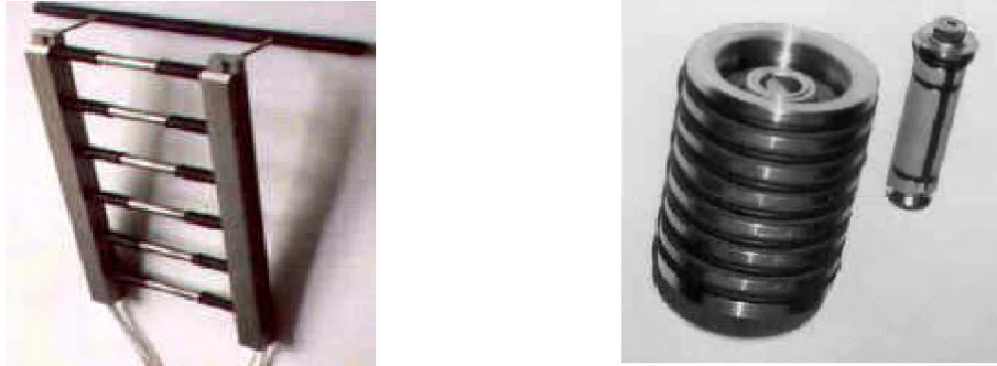
Figure 4. Sketch of the ladder macro-cell system (Broomfield (1997)).
