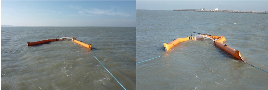
Figure 3: Towed Thomsea net. Left: normal conditions; right: net pushed out of angle by a strong sideways current (Zeebrugge West).
