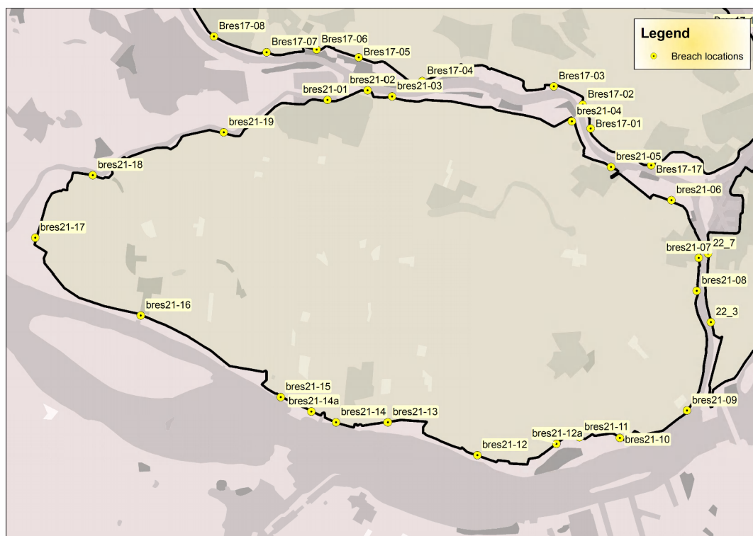
Figure 4.8 Investigated breach locations along dike ring 21 (Hoekse Waard)
