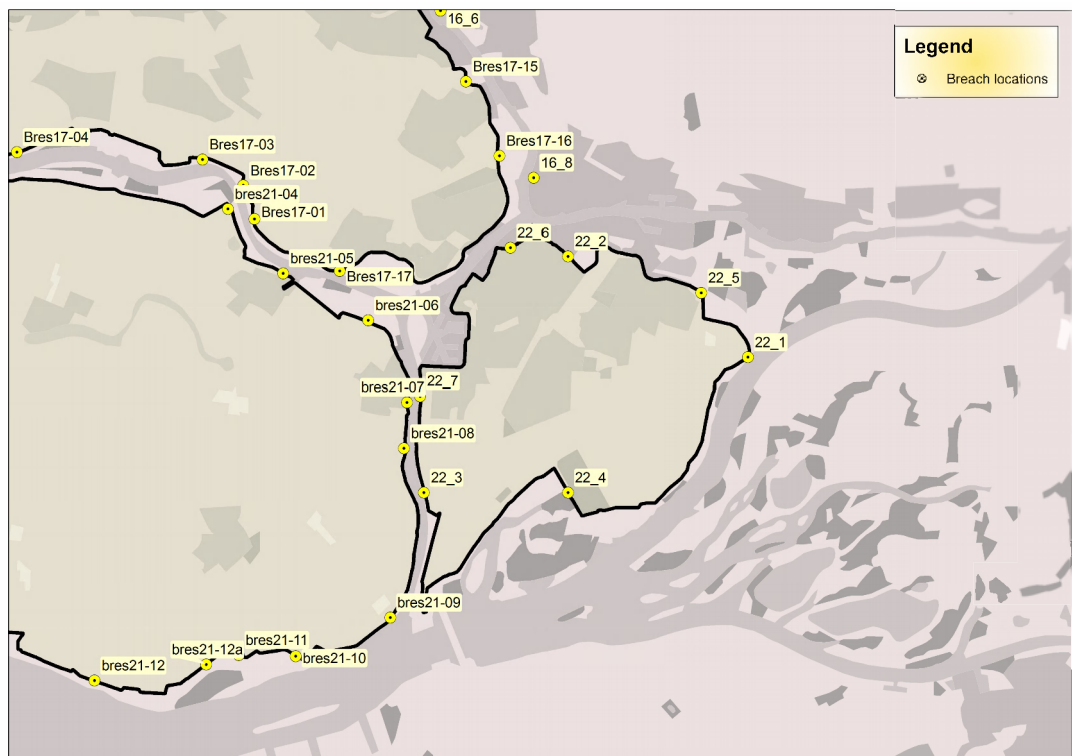
Figure 4.10 Investigated breach locations for dike ring 22 (Island of Dordrecht)
