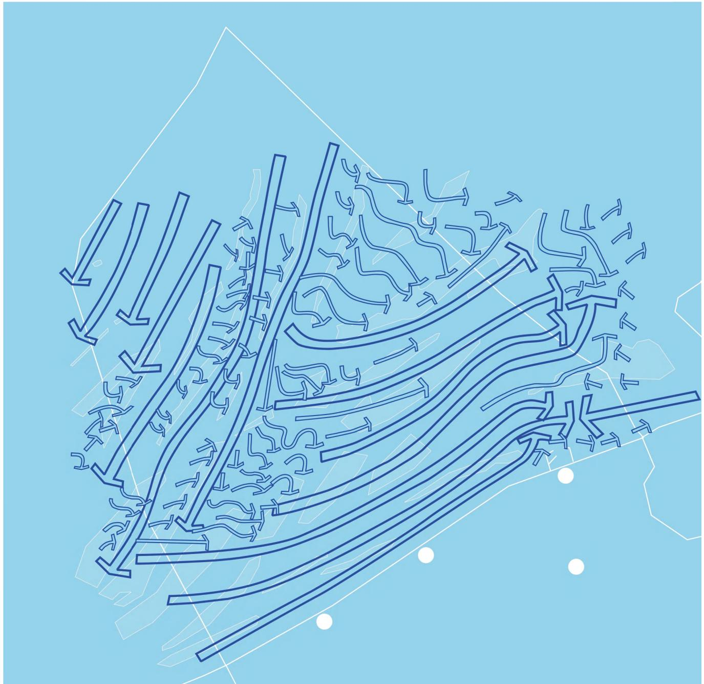
**Map III.1.1b. Conceptual view of the main sand transport directions on the seabed**
