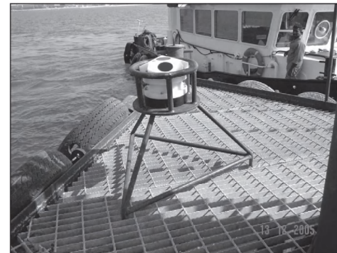
Picture 1: AWAC sensor and its mounting frame.
