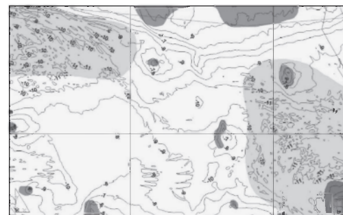
Figure 3: Fragment of the sedimentological interpretation (approx. 1200m by 750m) of the sonar mosaic shown in figure 2. Colours represent the sediment type.
