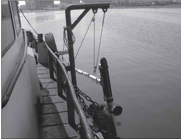
Photo 1: Side-scan sonar fish fixed at the extremity of a steel pole. Note the echosounder transducer attached to the sonar fish.
