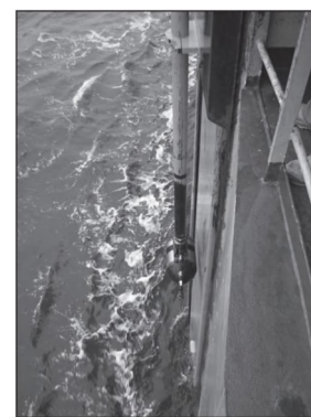
Photo 4: The Reson Seabat 8101 transducer attached to the extremity of a steel pole.
