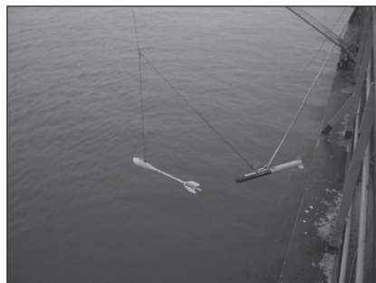
Photo 3: A 50kg lead weight made it possible to bring the sonar fish to a suitable depth while using a short length of cable.
