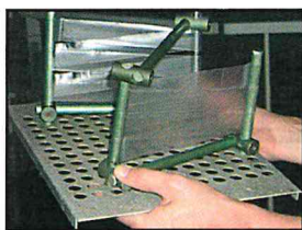
Semipermeable membrane devices, mounted for concentration measurements in water (top) and air (bottom).
