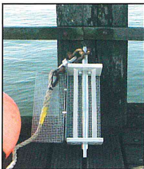
Semipermeable membrane devices, mounted for concentration measurements in water (top) and air (bottom).
