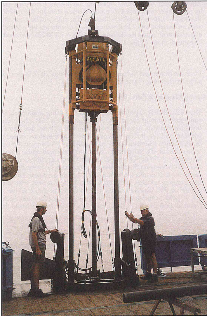
The vibrocorer during the ALW program 'Plume & Bloom'. Outcrops of Brown Bank Clay near East Anglia were mapped by this MRF-instrument. Photo: Martien Baars.
