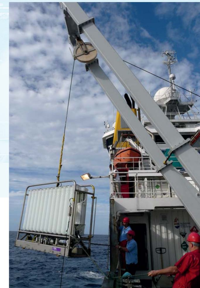
The titanium frame with 24 NIOZ developed 'pristine' ultra-clean water samplers is ready to be launched.
