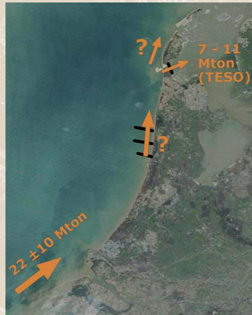
Satellite image of the Dutch coastal zone showing high suspended matter at the surface close to the coast in brown. The sediment transport direction and estimated volumes are indicated. Three black lines indicate the locations of the measurements.
