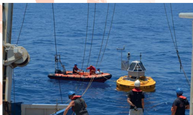
Recovering a TRAFFIC buoy that has collected Saharan dust for the past year.
