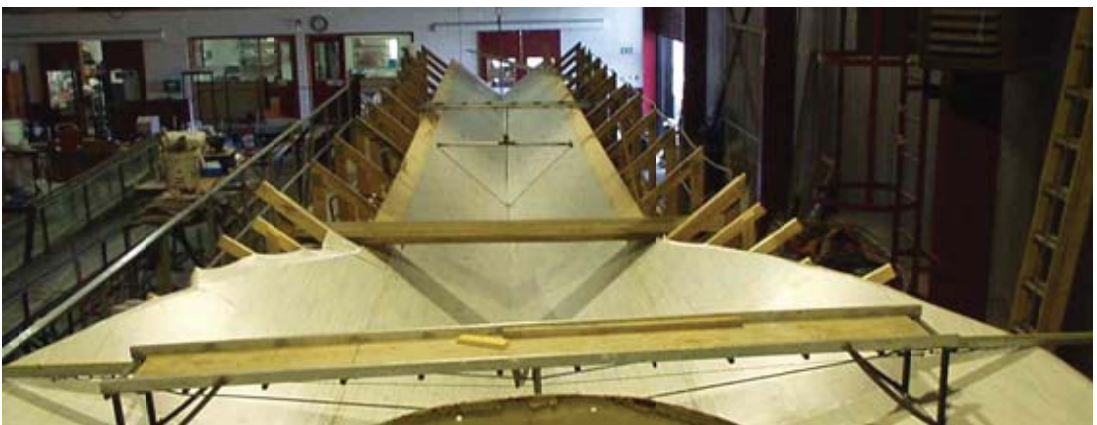
Figure 8.1 | Transition from pool to channel in a triangular flume. See Barnett, Painter and Watkins (2004).
