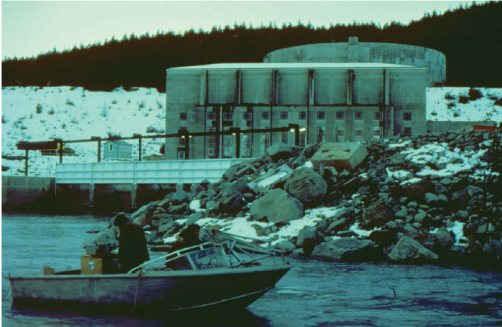
Figure 5.4 | Flow gauging using dye dilution sampling at the upstream end of hydropower canal.
