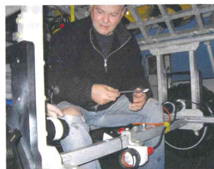
On board of NIOZ regional vessel RV Navicula NIOZ Instrument Technician Johan van Heerwaarden is adapting a video system on deep-sea crawler MOVE.
