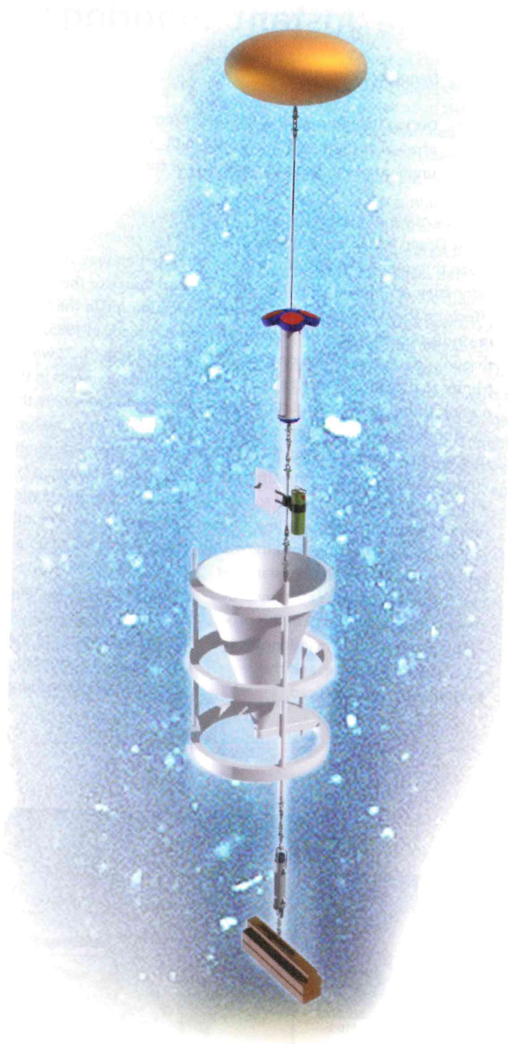
Schematic impression of a mooring. From bottom to top: Iron anchor weight, acoustic release, sediment trap, current meter, Acoustic Doppler Current Profiler (ADCP), and a sub-surface buoy to keep the mooring upright during the measurements and to lift it to the sea-surface after detachment from the anchor weight by means of an acoustic signal from the research vessel.
