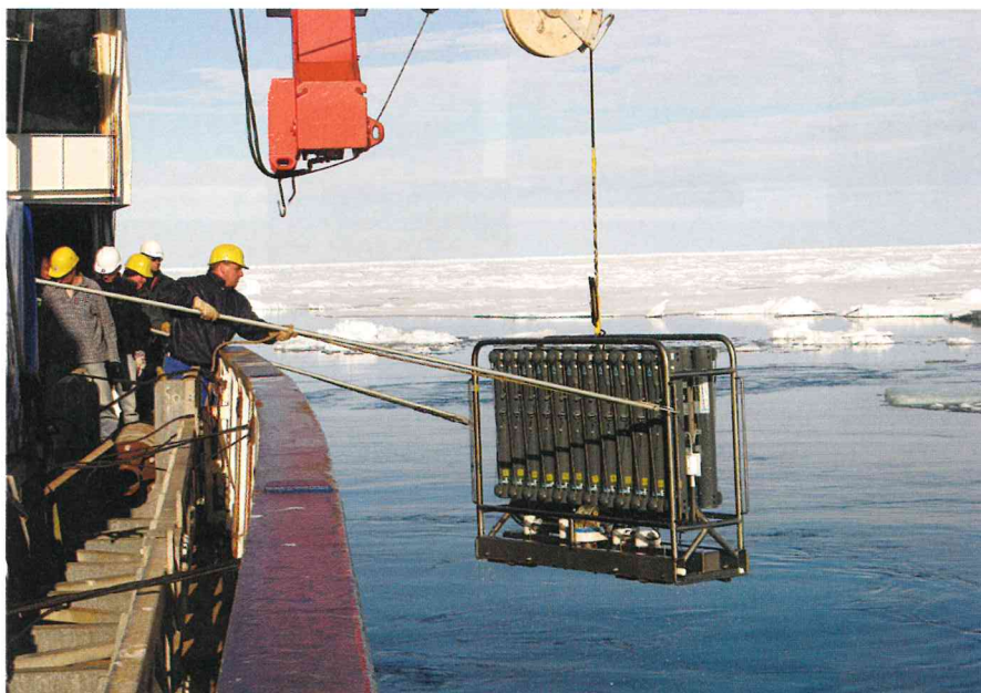
The Ultra Clean CTD alongside RV Polarstern during the ARK-XXII/2 cruise in the Polar Sea
