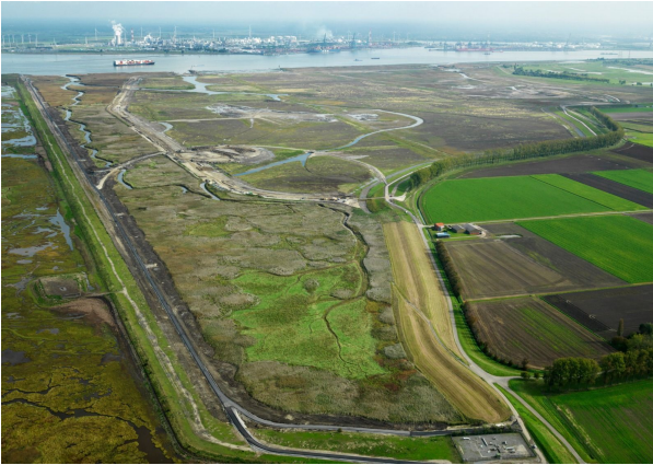
(a) A top view of the Hedwige-Prosperpolder after the opening in October 2022 during ebb tide. People dug several creeks to promote the area's natural development. Retrieved from Scheyen (2023, 25 mei).
