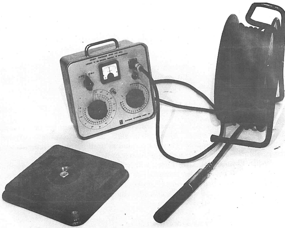
Fig. 6. Salinity temperature bridge (Electronic Switchgear MC5).
