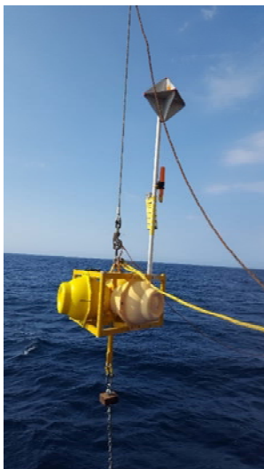
Buoy used to measure the ships sound away from the ship
