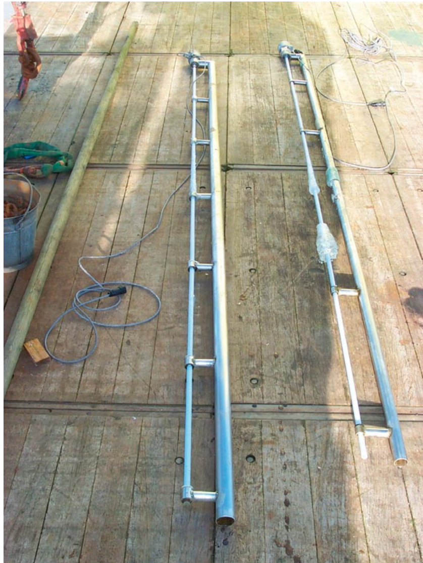
..... Photo 10 3-metre-capacitance probes FL5 (right, with some ice accretion) and FL9 (left), 23/1/2006
