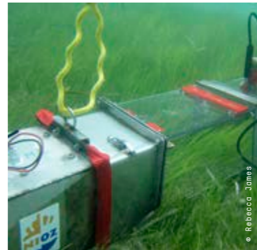
A PORTABLE WATER FLUME was used to measure sediment stabilisation.
