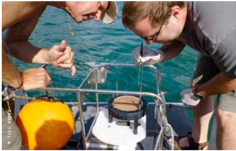
BACTERIA and other particles from Lake Lugano were collected on a glass fibre filter.
