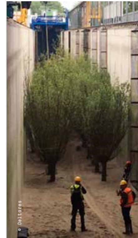
DURING THE WOODS VERSUS WAVES-EXPERIMENT , willows were positioned in the large Ducth Delta Flume to put the protective power of woods to the test.
