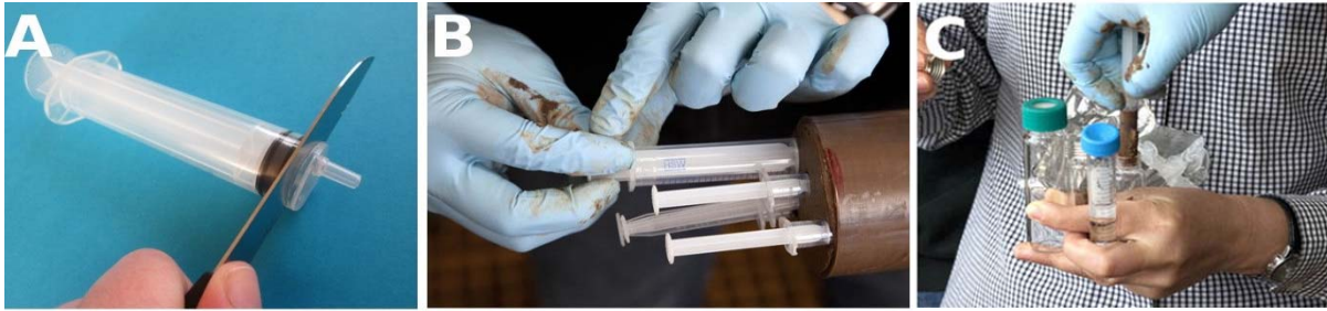
Figure 8.6. Subsampling of typical core for microbiology. All provided sampling material is sterile and ready to use. Sub-cores are taken ideally from the middle of the original core and transferred immediately to sterile plastic tubes (50 mL Falcon tubes) (C). The samples are then stored and transported as described for further analyses.
