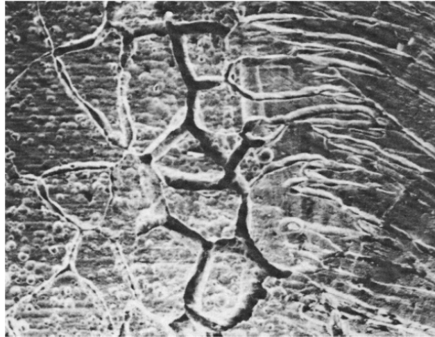
Figure 3-4 Intergranular corrosion in stainless steel[2].
