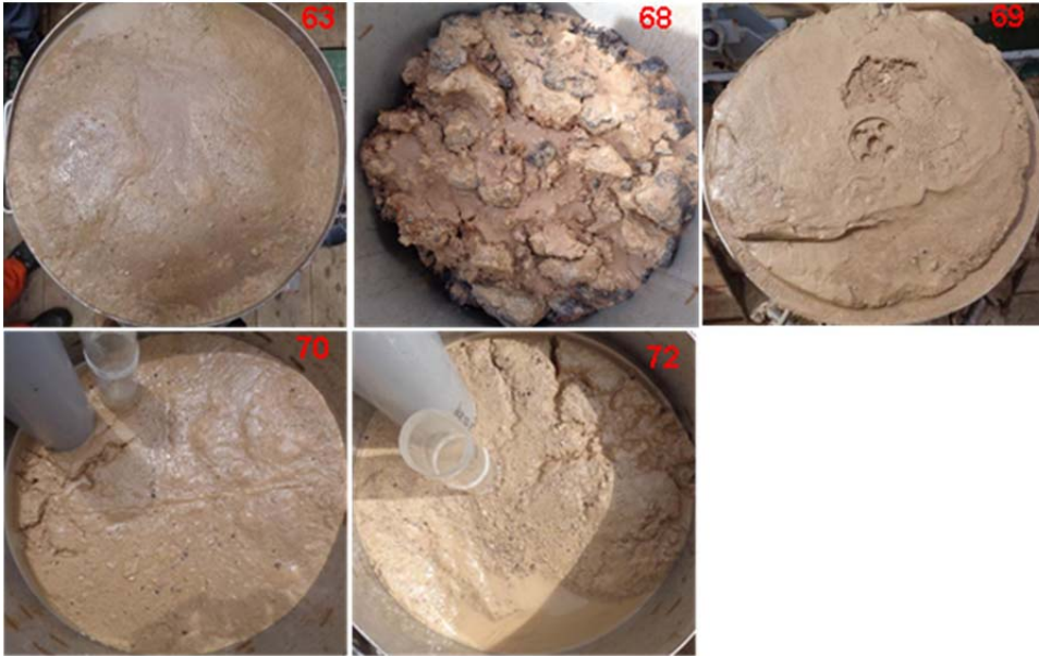
Figure 6.5. Surface pictures of the 5 boxcore samples after draining the overstanding water. Diameter of the core is 50 cm. Station numbers are indicated in red.
