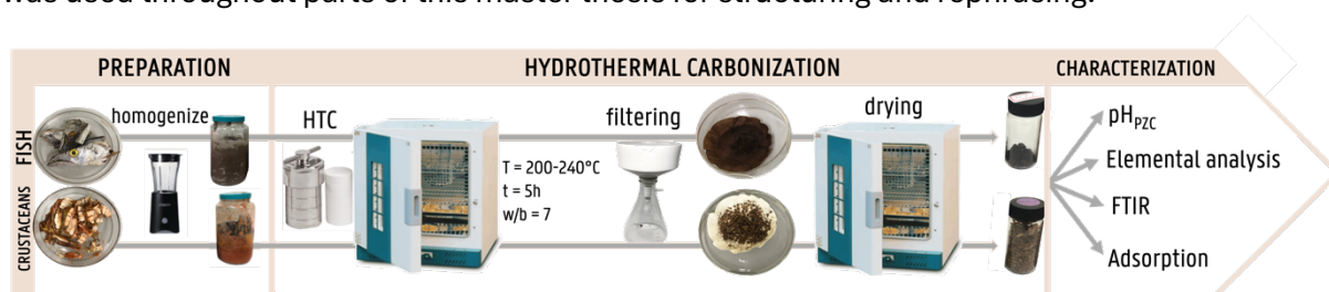
Figure 15: Schematic overview of feedstock preparation, HTC and hydrochar characterization.
