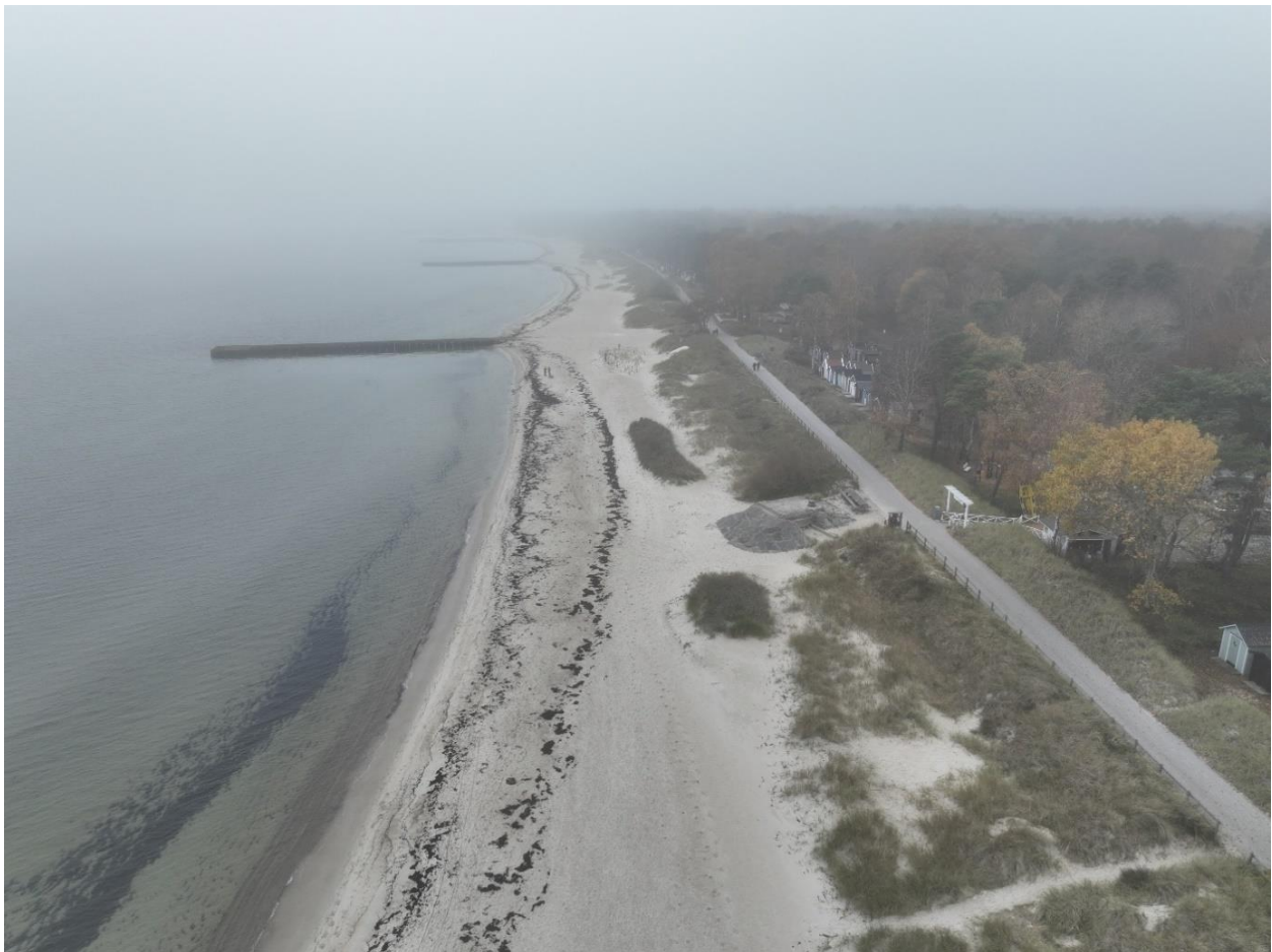
Figure 22 - Ystad (SE) Demonstrator, Dune-in-front-of-Dike
