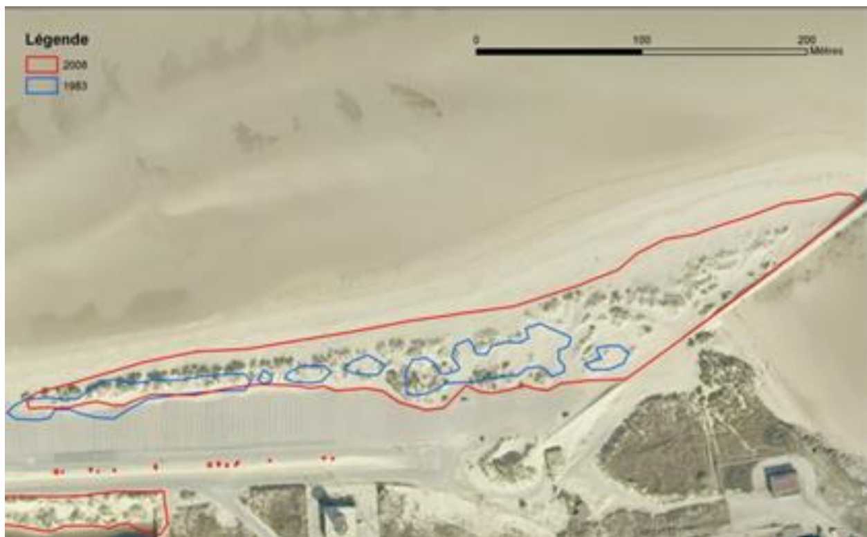
Figure 11 - 1983 and 2009 dune development at the toe of Digue du Break East (Tresca et al., 2014)
