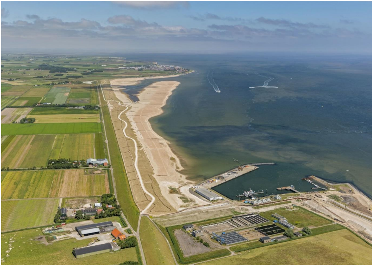
Figure 20 – Texel, Prins Hendrikzanddijk (NL) Demonstrator, Dune-in-front-of-Dike
