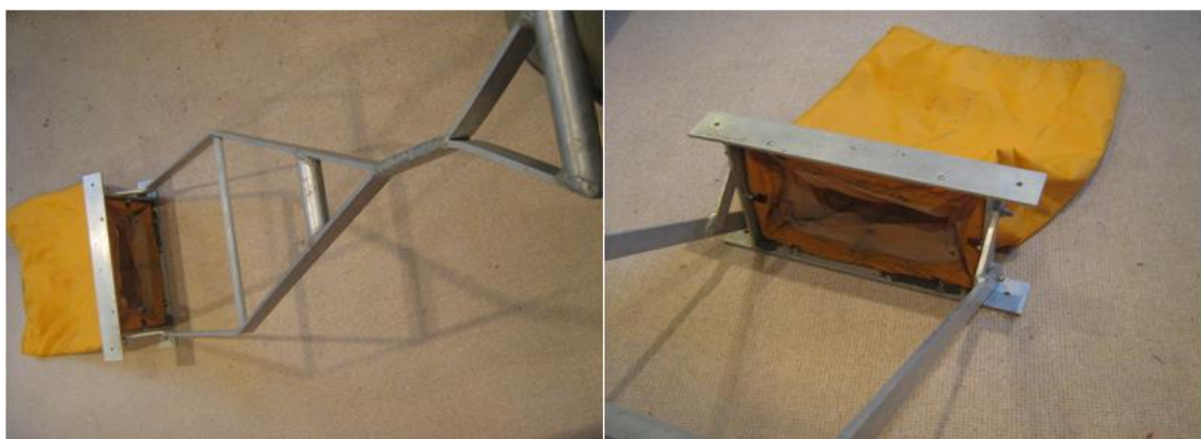
Figure 3.3: The hand held dredge designed to work in shallow water on the Holton Mere mudflat. The opening of the dredge is 30cm wide and the bag has a mesh size of 1mm. The dredge is pulled through the sediment for a distance of 1m in order to collect quantitative samples.
