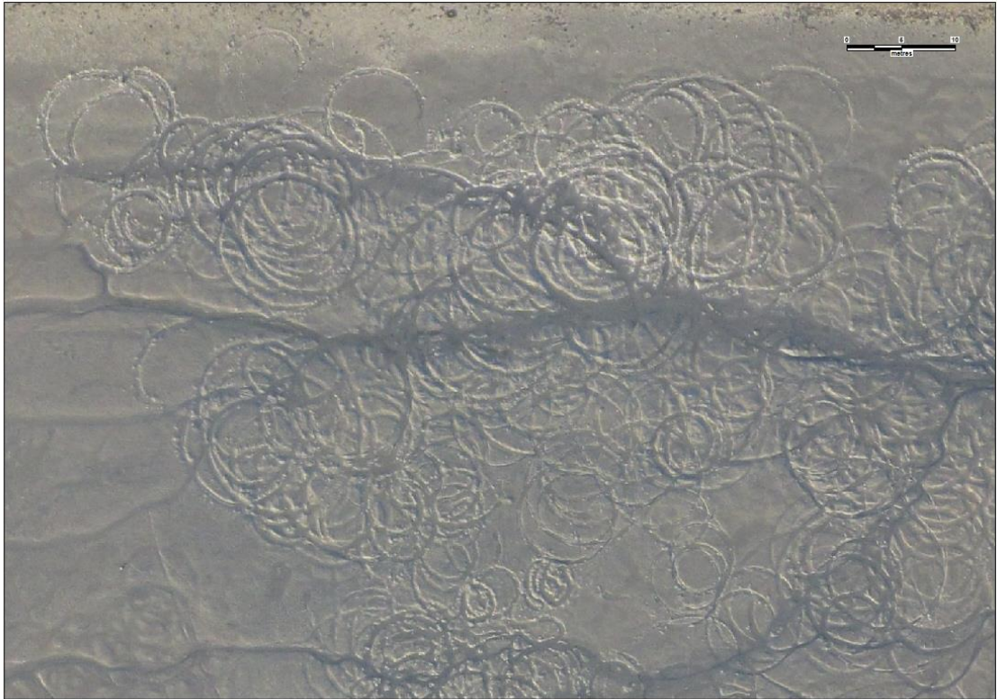
Figure 3.19: Aerial photograph of the effects of pump scoop dredging in Poole Harbour, image courtesy of Dorset Wildlife Trust. The round circles are the scars left from pump scoop dredging, the area of fishing is 90m by 60m, this highlights the intensity of the fishing effort.
