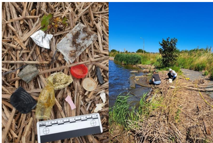
Figure 5: Macrolitter sampling using a transect method and the JRC App at the Yser riverbanks (Photos by Therese Nitschke, VLIZ).
