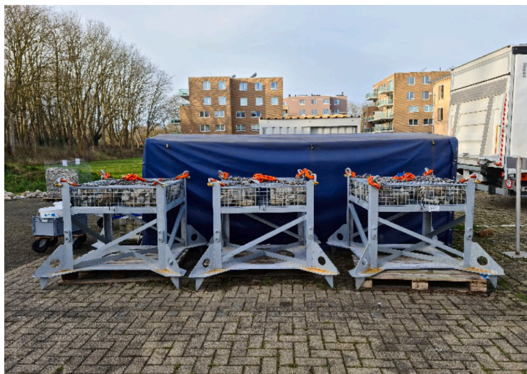
Fig. 2. The three stainless-steel units (1x1x1.4 m, left panel) used to test the effects of different habitat complexity treatments. The units were composed of a metal supporting structure and a one-by-one meter grid container of 20 cm height that was subdivided into four 45x45x20 cm compartments, allowing for 10 cm space between each compartment (right panel). The top of the table was covered by a 1x1m cover with a 2 × 2 cm mesh (not pictured here).
