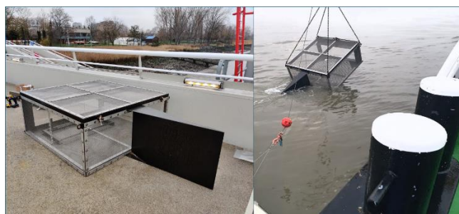
Figure 4: Left: The Bedload Sampler with the 1m long fin at the back of the cage (CREDIT: Remi Chevalier, UA). Right: The Bedload Sampler being lowered into the water at an angle of 30° (CREDIT: Mattias Bossaer, VLIZ).
