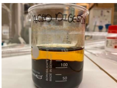
Figure A2.5 LHA solution after 24 hours of extraction using 12 M HCl.
