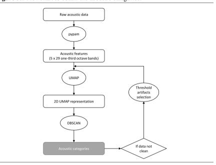
Figure 5.2 Flowchart to obtain the acoustic categories.
