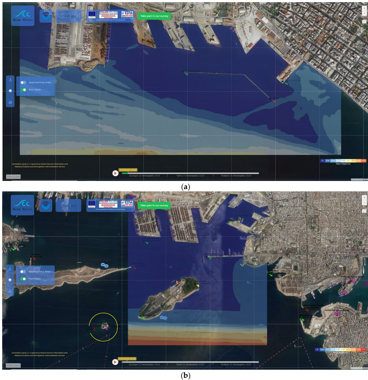
Figure 13. Final output version (provided freely) of the Accu-Waves WFS on the web-GIS app: illustration of Model B forecasts for 2-D horizontal fields of characteristic wave height ( H_s ) in the ports of (a) Thessaloniki, and (b) Piraeus (Aegean Sea, Mediterranean; upper and lower graphs, respectively) in January 2023.
