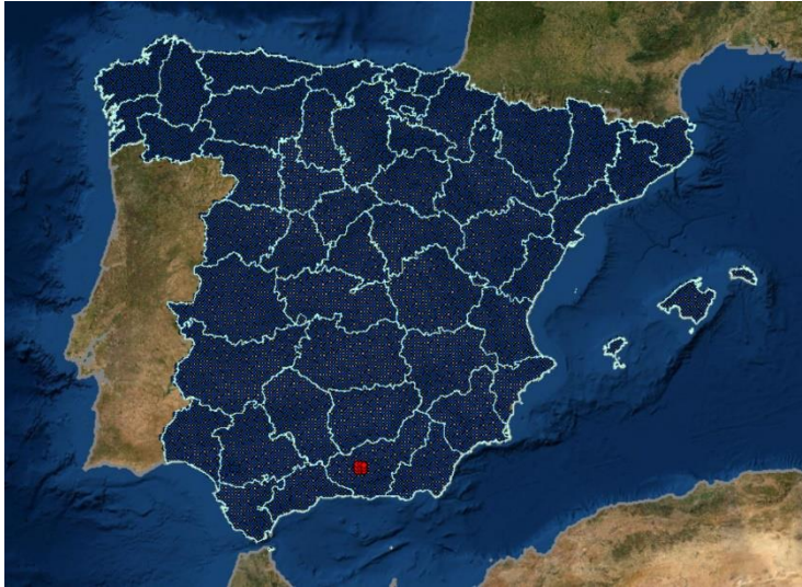
Figure 4.6. AEMET gridded model of high resolution (5x5 km) and the location of the 9 data points (red points) for estimating the average precipitation and temperature for the period 1951-2020 near the city of Granada.
