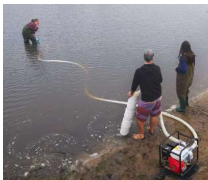
Figure 2. Pump sampling of surface waters, and filter column.
