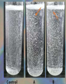
Figure 2. Bio flocculation activity of supernatant Gloecapsa sp. (A) and Gloecapsa sp. culture (B).
