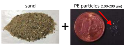
Fig. 1: sediment fraction (left) and polymer rich fraction (right) mass of polymer rich fraction 0.085 ± 0.022 % of artificial sediment
