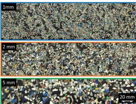
Fig. 2. Detail of the microplastic recovered from Playa Grande (Tenerife, Canary Islands, Spain) sorted by particle size.
