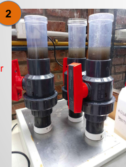
Fig. 2. MPs extraction with the Sediment Microplastic's isolation (SMI) unit..
