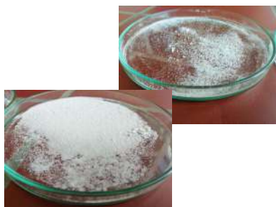
PE isolated from two personal care products (PE_PCPs_1 and PE_PCPs_2)
