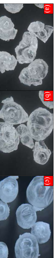
Figure 2. Microplastics swollen and pitted after 48-hour, 90°C digestions with (a) KOH, (b) NaOH and (c) H 2 O 2 at 2.5X magnification
