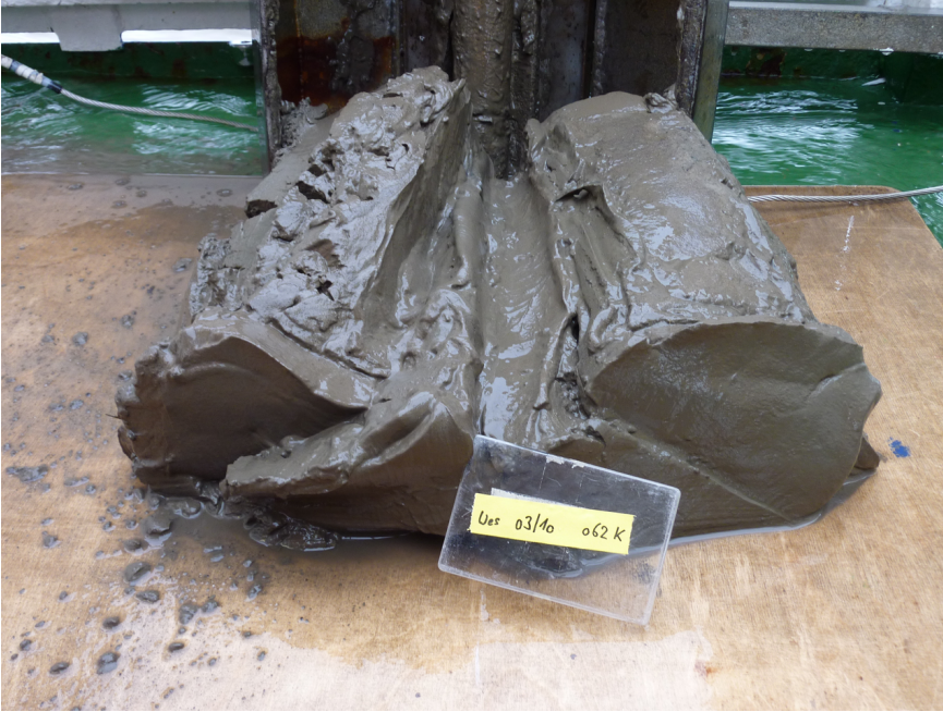
Figure 1.4: Consolidated mud sampled in the Weser estuary. Picture copied from https://de.wikipedia.org/wiki/Fluid_Mud , on 28/09/2023
