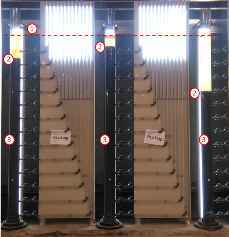
Figure 3.5: Setup of mud settling experiments performed at FH. Bright light panels illuminate the columns from behind, accentuating the water-mud interface. (1) Initial mud level; (2) settled water-mud interface; (3) mud column.
