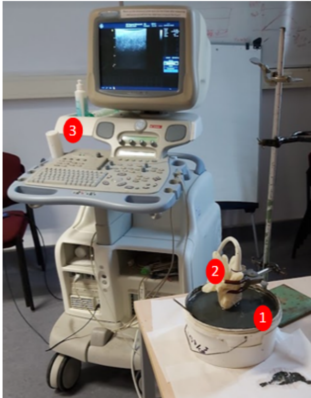
Figure 3.18: Setup of performed B-mode scan on mud: (1) bucket of mud with density 1.13 \text{ g}\cdot\text{cm}^{-3} , (2) 10L linear ultrasound array protected in a latex glove, (3) GE Vivid 7 ultrasound scanner. Apart from the array being immersed partly in the mud, the setup is in line with Fig. 3.1 (B).
