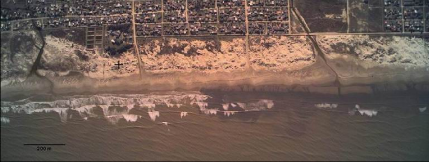
Figure 1.3: 1998 Airborne Data Acquisition and Registration (ADAR) image showing differential wave breaking due to shallow water mud deposits. The dark mud deposits are visible on the right half of the coastline captured in the image (Holland et al., 2009).
