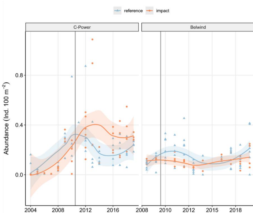
Figure 3.4: Plaice abundance in beam trawl samples (approx. 200 m from the turbines) for C-Power and Belwind in reference and impact areas over resp. the time span 2004-2019 and 2008-2019 4 . Vertical dark grey lines indicate the before and after construction period as considered in this study, which also coincides with the moment that fisheries activities were suspended for the second and third phase of C-Power and Belwind. The area around the 6 GBFs in C-Power (first construction phase) was closed in 2008. LOESS-smoothers with a span of 0.7 were fitted to the data to facilitate interpretation. Orange and blue bands indicate the standard error 95% confidence intervals for the impacted and reference areas, respectively.
