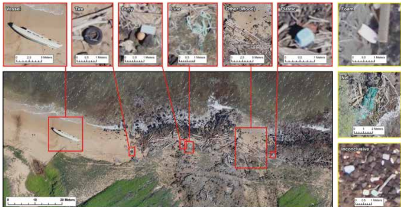
Figure 6-1 (below) Sample swath of coastline and the variety of debris identifiable in the high-resolution imagery. Items on the right (yellow outline) were found elsewhere and are included to demonstrate examples of the other debris types (from Moy et al., 2018).
