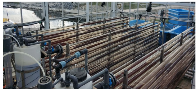
Fig. 1 Tubular photobioreactors located in Vlissingen and operated with R. salina
