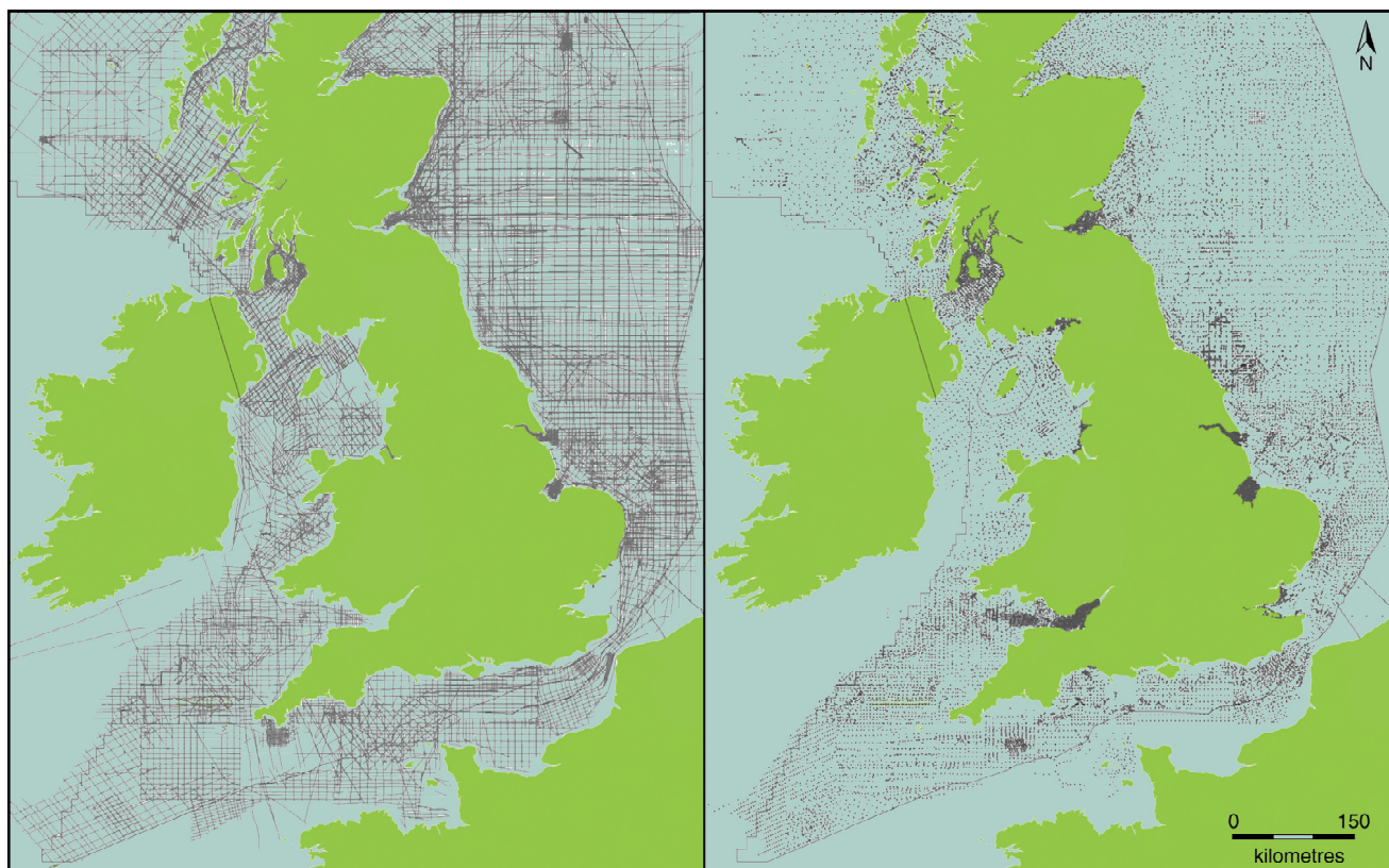
Figure 2.1 BGS survey coverage on the UK continental shelf as displayed by GeoIndex, October 2006. (a) shows geophysical profile lines, (b) shows shallow sediment sample stations
