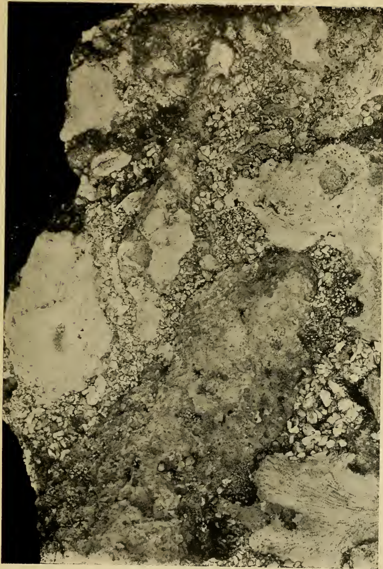
PHOTOGRAPH OF A FRACTURED SURFACE OF A PIECE OF BARRIER-FLAT BRECCIA, TO SHOW THE INCLUSION OF SMALL PARTICLES AND THE CEMENTING OF THE WHOLE MASS.
