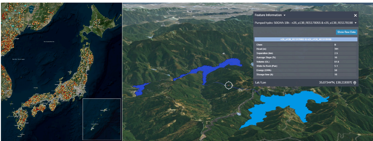
Fig. 7. Distribution of off-river pumped hydro sites in Japan (left) and 3D visualization of a sample site in Chubu (right). Image from Australian Renewable Energy Mapping Infrastructure [72] and original data from the Australian National University Global Pumped Hydro Atlas [26].
