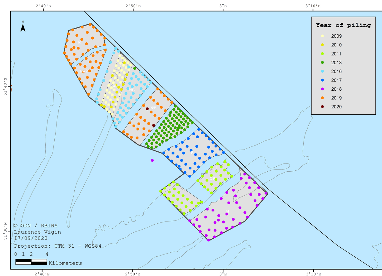
Figure 1. Timing and location of pile driving events in the Belgian part of the North Sea (period 2009-2020, data RBINS). From 2013 onwards, a seasonal pile driving ban from January 1 st to April 30 th was enforced. From 2017 onwards developers were obliged to use noise mitigation measures that limit the transmission of noise pollution to the marine environment.
