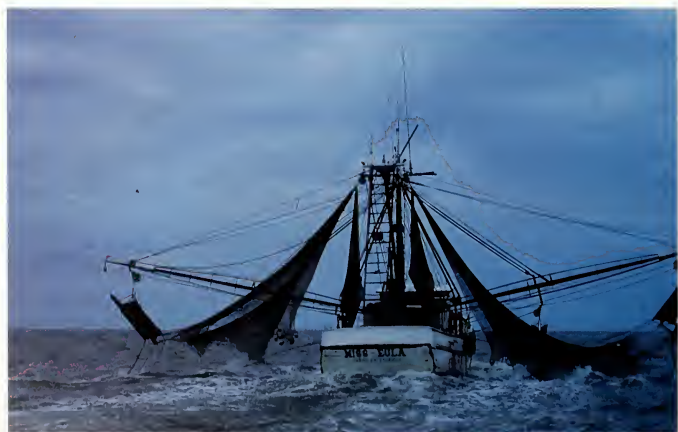
TOP: Native Americans in the 1950s work from wooden platforms on the Columbia River to take returning salmon. Scientific Publications Unit, NOAA Fisheries. CENTER: Steel “doors” hung on the stern of this moored vessel in Santa Barbara, California, advertise its use as a trawler. William B. Folsom, NOAA Fisheries. BOTTOM: The distinctive Gulf of Mexico shrimper prepares to lower its twin side-trawls off Alabama. William B. Folsom, NOAA Fisheries
