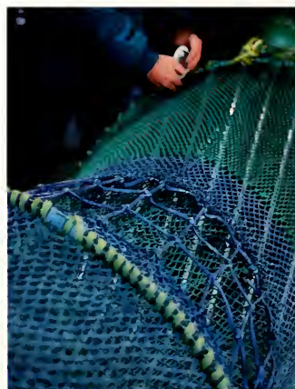
TOP LEFT: A trawl net rigged for fishing on the sea floor. INSET: Detail of trawl net with bycatch-reduction device. Jim Bean, Communications Collective/NOAA Fisheries. TOP RIGHT: A shrimp trawl net is readied for a trip out of Biloxi, Mississippi. William B. Folsom, NOAA Fisheries. BOTTOM RIGHT: A netmaker puts the finishing touches on a shrimp net equipped with devices to reduce bycatch and exclude sea turtles. William B. Folsom, NOAA Fisheries. BOTTOM LEFT: Welders work at night on an iron scallop dredge to ready it for the next day's fishing. © Nance S. Truworthy
