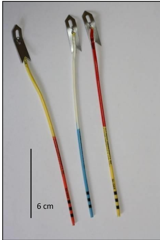
Figure 3.2: Hallprint Stainless Steel Dart Tags used to identify tagged sevengill sharks.
